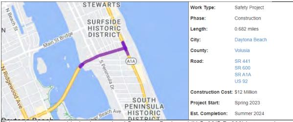
This project involves widening International Speedway Boulevard (U.S. 92/S.R. 600) between the Halifax River Bridge and S.R. A1A to provide two travel lanes, a 6-foot-wide sidewalk headed westbound, and a 10-foot-wide sidewalk headed eastbound. Improvements also include resurfacing along International Speedway Boulevard, building a raised median, and upgrading the traffic signals at Halifax Avenue, Peninsula Drive (S.R. 441), Grandview Avenue and S.R. A1A.
