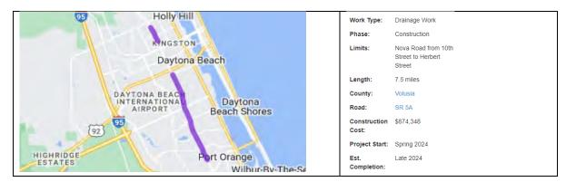
The purpose of the project is to restore the Nova Canal drainage system along Nova Road (S.R. 5A) from 10th Street to 3rd Street and Orange Ave and Canal View Blvd. / Herbert St. Work includes cleaning, reshaping, clearing & grubbing, tree and vegetation removal, herbicide application, and turf restoration in a series of canal segments.
