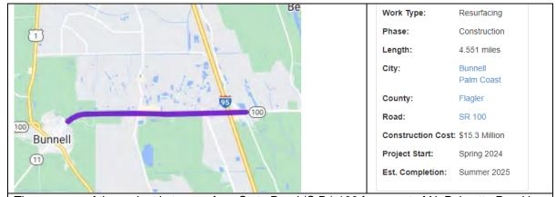
The purpose of the project is to resurface State Road (S.R.) 100 from east of N. Palmetto Road in Bunnell to east of Old Kings Road in Palm Coast to extend the service life of the existing roadway. Improvements include constructing 6-foot-wide sidewalk to close sidewalk gaps where existing right of way allows and improving pedestrian features at intersections within the project limits. The
